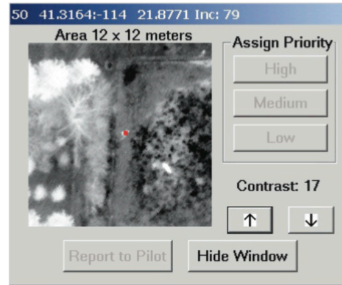
High resolution thermal thumbnails (brighter pixels=warmer temperatures, darker=cooler)
